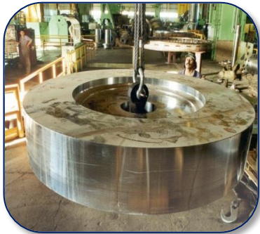
Disco forjado D=3100mm H=680mm
